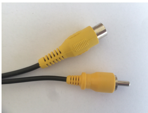
Obr. 3: RCA pin jack
